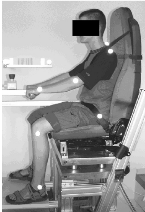
Fig. 1. A male subject sitting in the upper part of the seat, mounted on a Kistler force plate.
